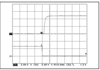
Figure 10: Turn-on transient at zero load (10 ms/div). Ch 1: Vout (5V/div) Ch 2: ON/OFF input (5V/div)
