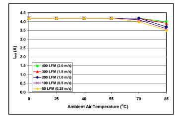
Figure 5: Maximum output power derating curves vs. ambient air temperature for airflow rates of 50 LFM through 400 LFM with air flowing across the converter from pin 3 to pin 1 (nominal input voltage).
