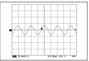
**Figure 16:** Output voltage ripple at nominal input voltage and rated load current (50 mV/div). Load capacitance:  $1\mu$ F ceramic capacitor and  $10\mu$ F tantalum capacitor. Bandwidth: 20 MHz. See Figure 13.
