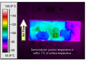
Figure 6: Thermal plot of converter at 4.2 amp load current (50W) with 55°C air flowing at the rate of 200 LFM. Air is flowing across the converter from pin 3 to pin 1 (nominal input voltage).
