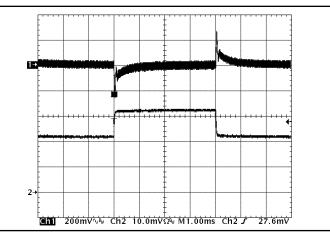
**Figure 11:** Output voltage response to step-change in load current (50%-75%-50% of Iout(max);  $dI/dt = 0.1A/\mu s$ ). Load cap:  $10\mu F$ ,  $100 \text{ m}\Omega$  ESR tantalum capacitor and  $1\mu F$  ceramic capacitor. Ch 1: Vout (200mV/div), Ch 2: Iout (1A/div).
