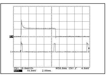
**Figure 18:** Load current (5A/div) as a function of time when the converter attempts to turn on into a 10 m $\Omega$  short circuit. Top trace (2.0ms/div) is an expansion of the on-time portion of the bottom trace.
