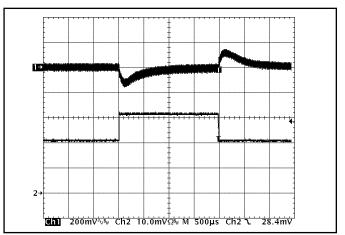
**Figure 12:** Output voltage response to step-change in load current (50%-75%-50% of Iout(max):  $dI/dt = 5A/\mu s$ ). Load cap:  $470\mu F$ ,  $30 \ m\Omega ESR$  tantalum capacitor and  $1\mu F$  ceramic cap. Ch 1: Vout (200mV/div), Ch 2: Iout (1A/div).
