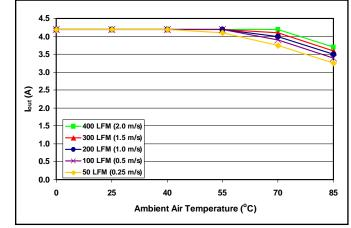
Figure 7: Maximum output power-derating curves vs. ambient air temperature for airflow rates of 50 LFM through 400 LFM with air flowing from input to output (nominal input voltage).
