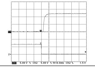
**Figure 9:** Turn-on transient at full load (resistive load) (10 ms/div). Input voltage pre-applied. Ch 1: Vout (5V/div); Ch 2: ON/OFF input (5V/div)
