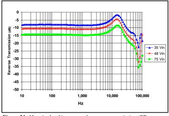
**Figure 21:** Magnitude of incremental reverse transmission ( $RT = i_{in}/i_{out}$ ) for minimum, nominal, and maximum input voltage at full rated power.
